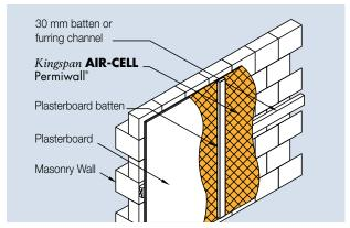
Figure 3  $\it Kingspan$  AIR-CELL  $\it Permiwall^*$  counter-batten system
