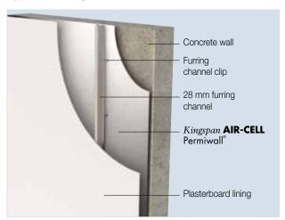
Figure 1 Kingspan AIR-CELL Permiwall® clip-and-channel system
